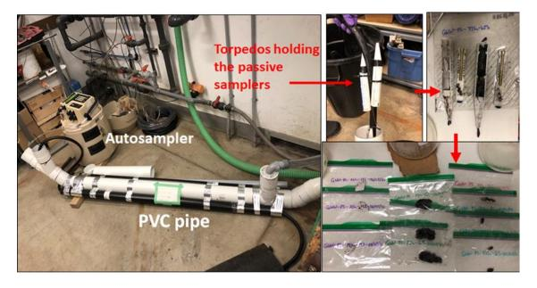
Fig. 3 Experimental Set-up of COVID-19 Wastewater Research
