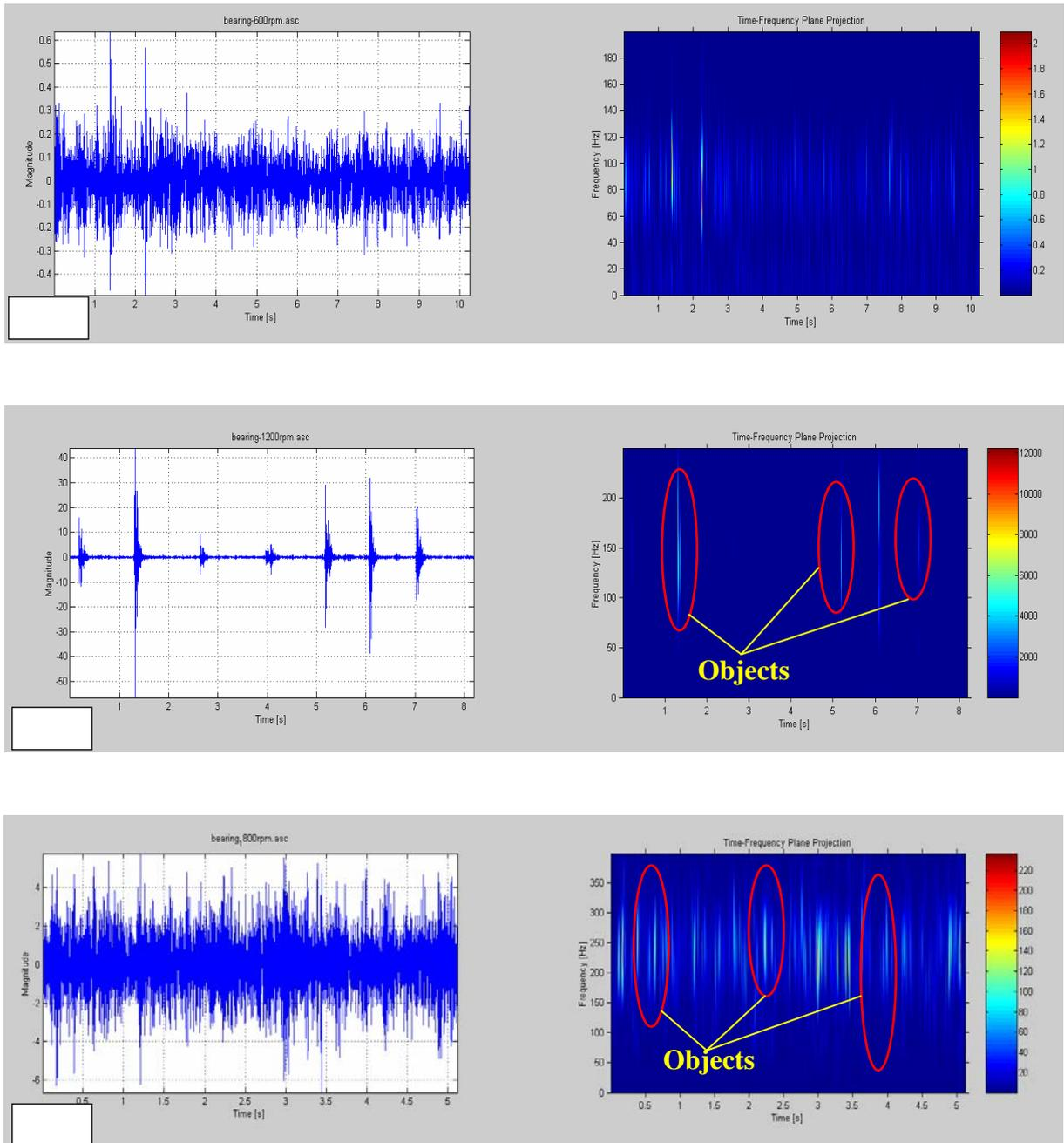
**Fig.9** STFT image of the simulated Ball fault class at a) 600 rpm, b) 1200 rpm and 1800 rpm.
