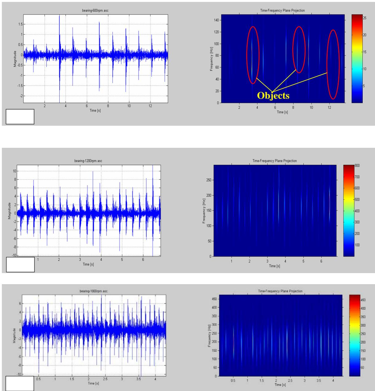
**Fig.11** STFT image of the simulated Outer fault class at a) 600 rpm, b) 1200 rpm and 1800 rpm.
