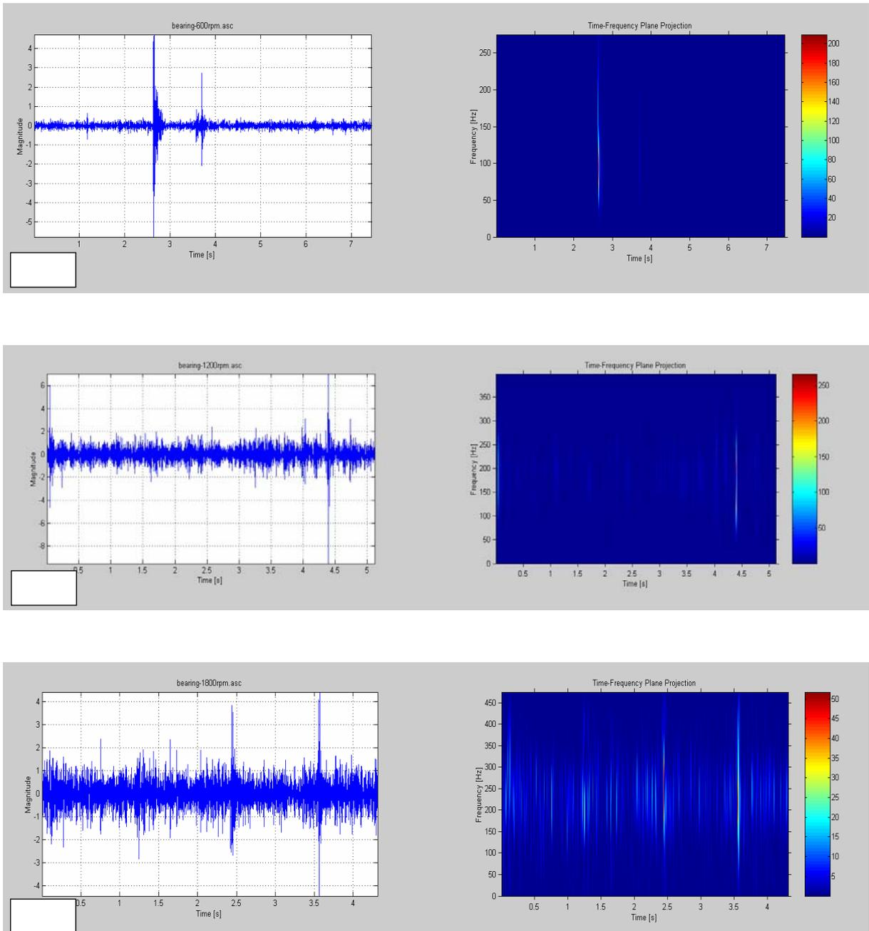
**Fig.10** STFT image of the simulated Inner fault class at a) 600 rpm, b) 1200 rpm and 1800 rpm.
