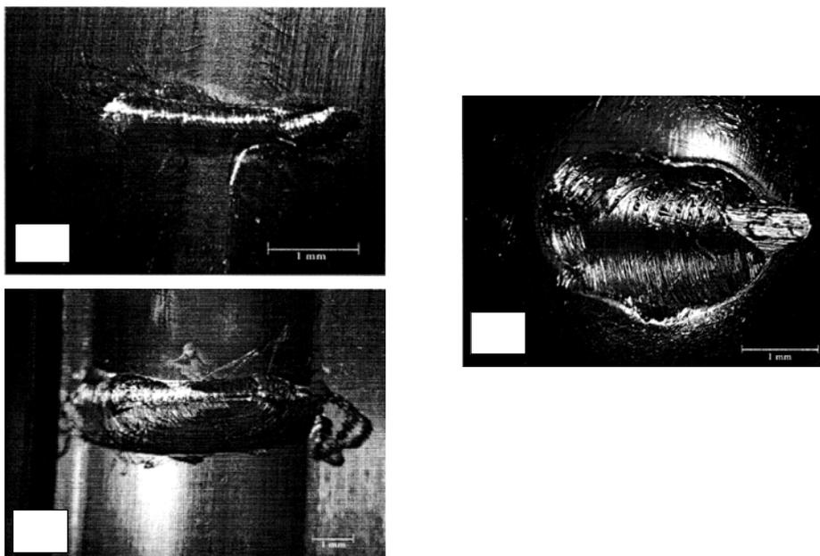
**Fig.7** Fault simulations on SKF 1211bearing a) outer race fault, b) inner race fault and c) ball fault.
