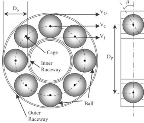
Fig.5 Dimension and frequencies related to bearing faults signatures.
