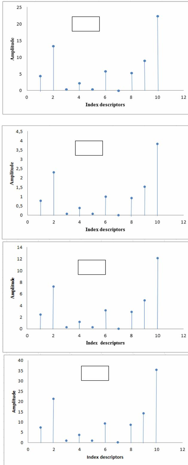
**Fig.12** Fourier descriptors of one object of STFT image at 600 rpm of : **a)** Normal class **b)** Defect ball **c)** Inner race defect **d)** Outer race defect.
