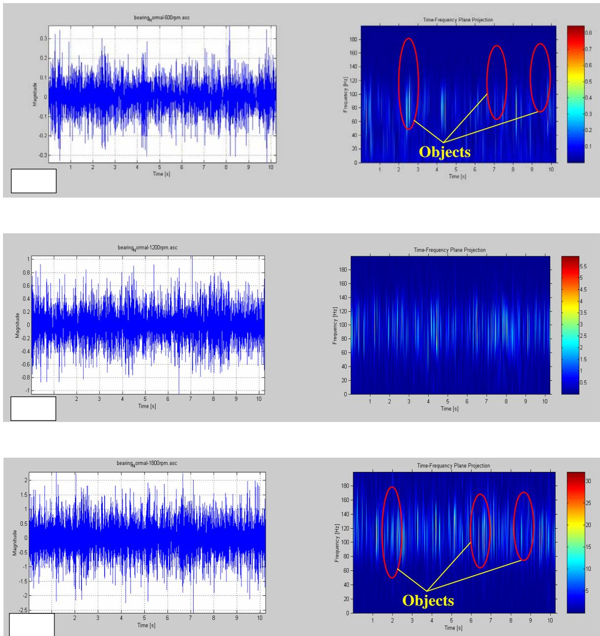
**Fig.8** STFT image of the simulated Normal class at a) 600 rpm, b) 1200 rpm and 1800 rpm.
